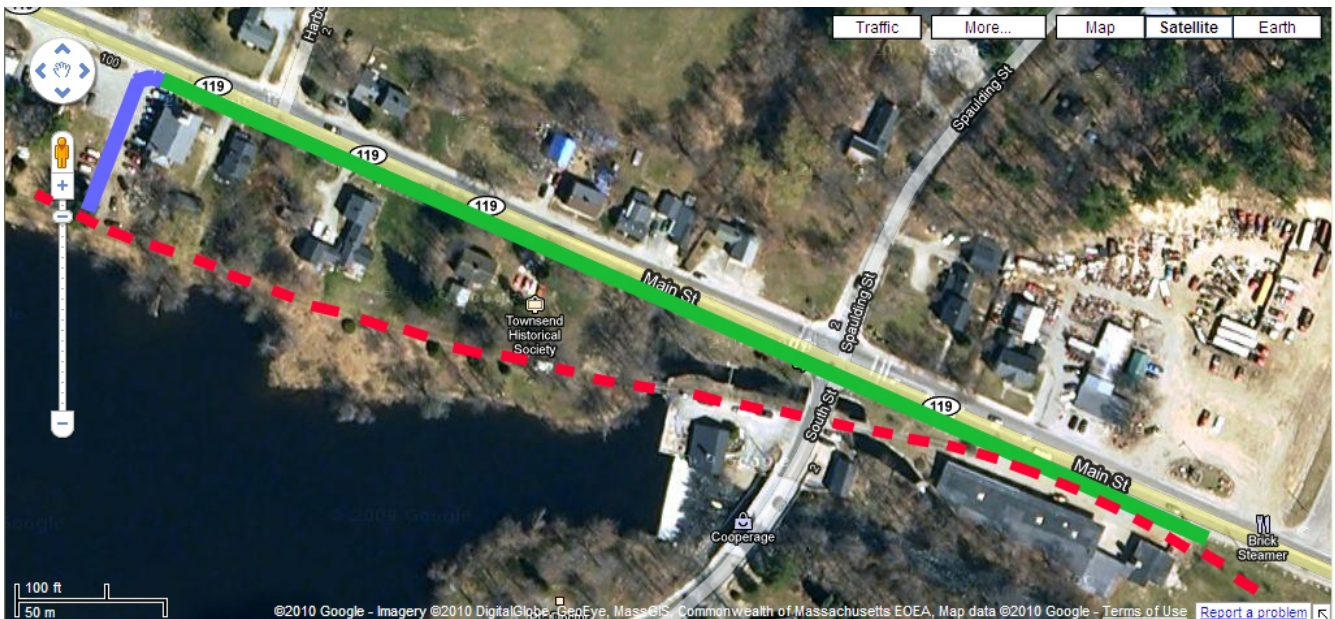
Figure 2: Sidewalk and rail bed alternative routes. Green: proposed sidewalk. Blue: return to rail bed via Harbor Church parking lot. Red dashed line: MBTA rail bed.
